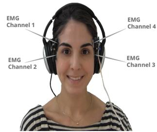
Fig. 2. Wearable used to measure distal EMG from four channels placed on the sides of the face, on both temples of the head. This configuration enables facial expression identification without obstructing the face. However, this makes identifying which muscle produced the measured activity challenging.
