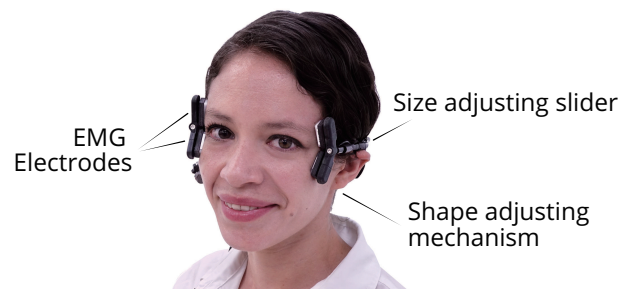
Figure 1: The wearable device used to record EMG during the elicited smiling behavior.
